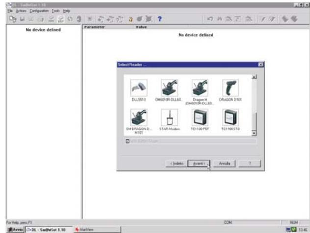
DL Sm@rtSet™ is supported by an easy-to-use graphic interface, based on Windows standards: Tree View on the left side and listing of all the configurable parameters on the right side. The action log has an Undo function, so any configuration mistake can be deleted. Furthermore, with DL Sm@rtSet™ it is possible to view all parameters that have been changed, so right away you can recognize them. All these characteristics make this program intuitive and instinctive to use.
